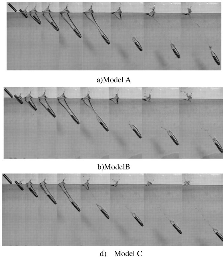
Figure 4. Inlet navigation attitude and bubble evolution chart at initial velocity of 2.63m/s.
