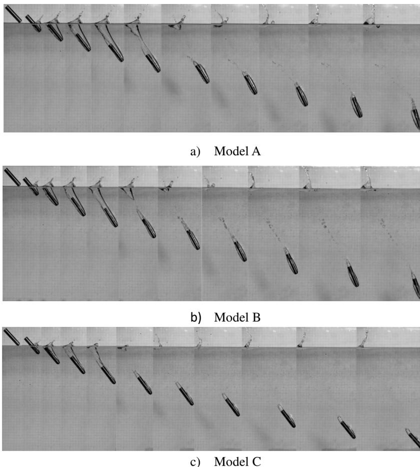
Figure 3. Inlet navigation attitude and bubble evolution chart with initial velocity of 1.95m/s.
