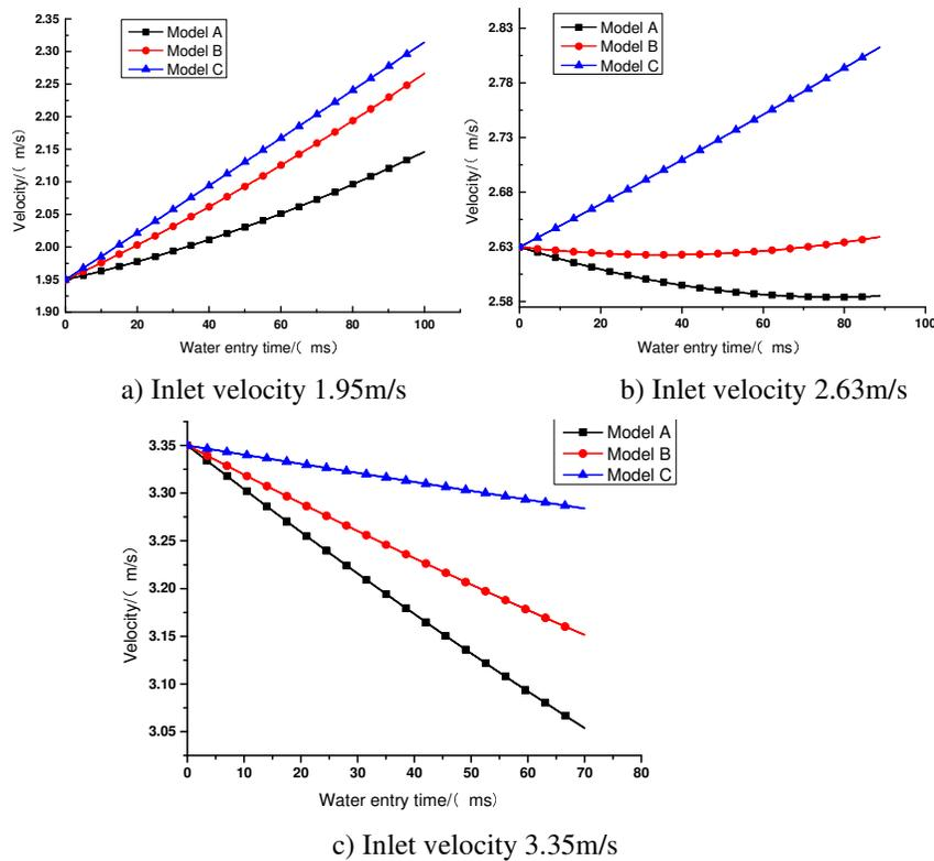
Figure 8. Velocity changes with time.
