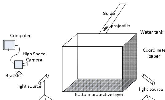
Figure 1. An experimental device for oblique water entry e.
