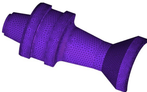
(b) Detailed surface mesh of one sabot petal
